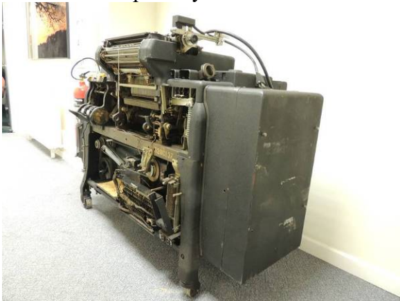
The 416 Tabulator stripped to door width
